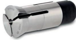
On MANURHIN K'MX 1032 SWING we use the guide bushes of type T229 denomination. We recommend the guide bushes with hard metal insert from renowned manufacturers.
