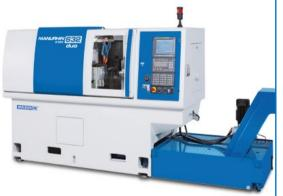
THE MANURHIN K'MX 632 DUO is designed for productive machining of parts for bars with a maximum diameter of 32 mm. With a spindle bore diameter of 37 mm, no modification of the end of the bar for bar feeder collet is needed. The machine comes standard with two electro spindles, each with a maximum speed of 10,000 rpm and with a rotary guide bush synchronized by pulleys and belts from the main spindle. Six linear CNC axes (X1, X2, Y1, Y2, Z1, Z2) and two rotary axes (C1, C2).
