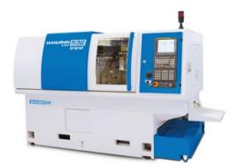
THE MANURHIN K'MX 532 TREND is designed for productive machining of parts for bars with a maximum diameter of 32 mm. With a spindle bore diameter of 37 mm, no modification of the end of the bar for bar feeder collet is needed. The machine comes standard with two electro spindles, each with a maximum speed of 10,000 rpm and with a rotary guide bush, synchronized by pulleys and belts from the main spindle. Five linear axes (X1, Y1, Y2, Z1, Z2) two rotary axes (C1, C2).
