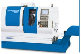
THE MANURHIN K'MX 816 CLEVER is designed for the productive machining of parts for bars of a maximum diameter of either 16mm or 20mm. The machine comes standard with two electro spindles and a rotary guide bush that is synchronized by pulleys and belts from the main spindle. Eight linear CNC axes (X1, X2, Y1, Y2, Y3, Z1, Z2, Z3) and two rotary axes (C1, C2) enable the machine to produce parts ranging in complexity. The construction solution enables the use of 4 tools at the same time.
